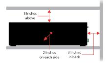
**CAUTION!** Do not block the ventilation holes on the sides and bottom of the
