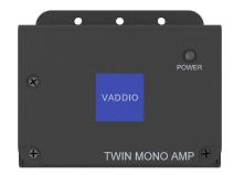
The Twin Mono AMP is an 8 Ohm 30 Watt mono power audio amplifier with a single differential input feeding two amplified outputs, each capable of driving into loads as low as 4 ohm. Ensure remote participants in small and medium conference rooms or classrooms are heard in collaboration and conferencing environments.
