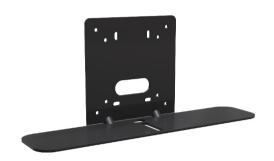
ADA-compliant thin profile wall mounting bracket for Poly Studio E70 with less than 4" protrusion from the wall with the camera attached. Easily mount to carts or monitor arms with the 75mm or 100mm VESA mounting patterns or connect to duplex electrical boxes with convenient leveling slots.
